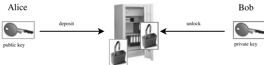
Fig. 6.3 Analogy for public-key encryption: a safe with public lock for depositing a message and a secret lock for retrieving a message
