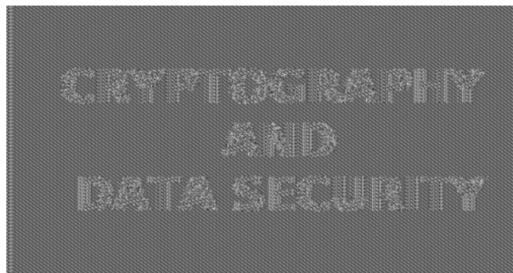
Fig. 5.3 Image and encrypted image using AES with 256-bit key in ECB mode
