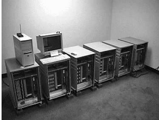
Fig. 3.15 Deep Crack — the hardware exhaustive key-search machine that broke DES in 1998 (reproduced with permission from Paul Kocher)
